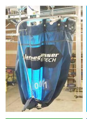
The **BAG ZAPPER** is automated and integrated into your rail system, cleaning bags after every use. No downtime, no labor involved, and a mere fraction of what the typical bag cleaning process costs.
